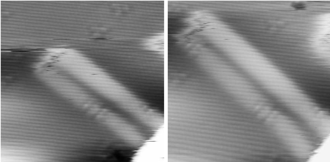
**Fig. 4.** Consecutive images showing the change in length (climb) of the dislocations. The image sizes are  $10\text{nm} \times 10\text{nm}$ . The time between images is 3 minutes.
