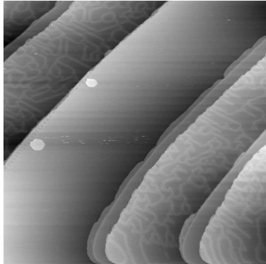
**Fig. 1.** STM image of a 1ML Cu film on Ru(0001). The image size is 284nm×284nm. Several substrate terraces, covered by the Cu monolayer, can be seen. On some, misfit dislocations are nucleated. Some of the terraces are bare of dislocations (and instead contain nucleated islands).
