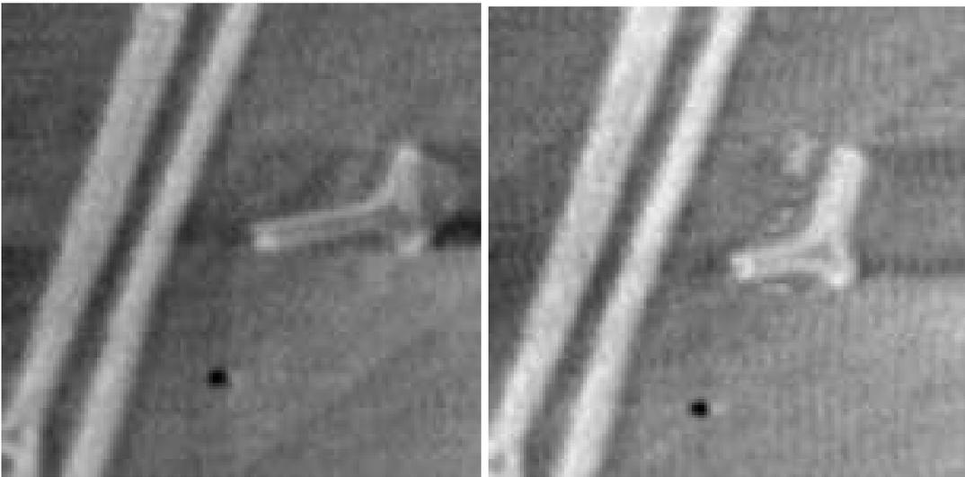
**Fig. 5.** STM images from a movie. A trigon which has undergone both climb and glide is shown in both images. The time interval between them is 20 minutes. The image size is 50nm×50nm.
