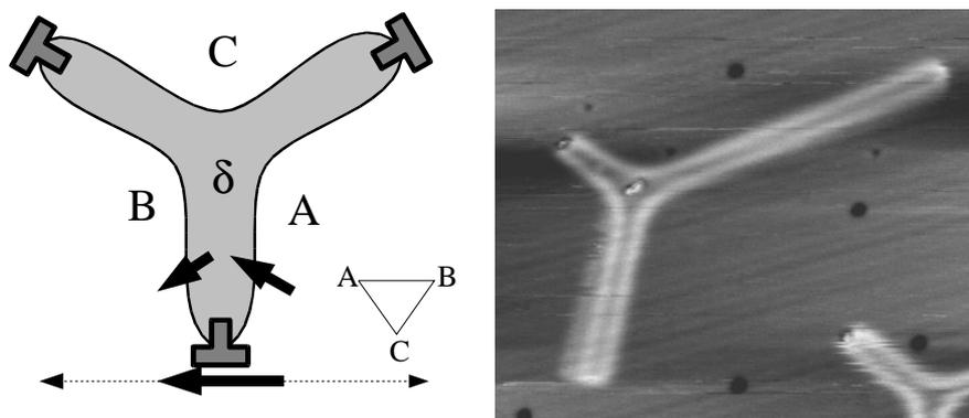
**Fig. 2.** Left: schematic of the structure of a trigon, showing the threading dislocations as small “T”s. The light grey area contains a stacking fault. The Thomson tetrahedron is also shown. The thick black arrows represent the Burgers vector of the dislocations. The glide direction for the BA dislocations is shown as a dotted line. Right: STM image (37.4nm ×32.4nm) of a trigon.
