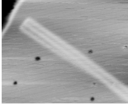
**Fig. 3.** STM image of dislocation glide. The image size is  $32.8\text{nm} \times 27.1\text{nm}$ . One end of the misfit dislocation is observed at two different positions.
