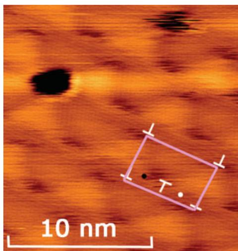
Fig. 8. STM image at 150 K of the initial S etching of SHB of Ag/Ru(0001) process showing two S-filled Ag vacancy islands. There are two equivalent etching sites per primitive unit cell, which are marked with black and white dots, each of the S-filled vacancies in the image residing on one of them. [Color figure can be viewed in the online issue, which is available at [www.interscience.wiley.com](http://www.interscience.wiley.com).]
