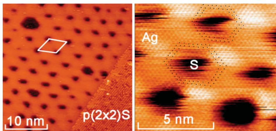
Fig. 7. S etching induced restructuring of the SHB of Ag/Ru(0001) ( $T = 295$  K): (right) no threading dislocations are left in the Ag film after S etching; (left) new triangular symmetry of the superstructure with S-filled vacancy islands 50 Å apart. [Color figure can be viewed in the online issue, which is available at [www.interscience.wiley.com](http://www.interscience.wiley.com).]
