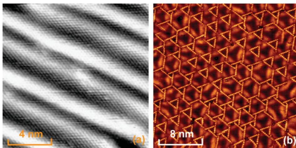
Fig. 9. Sulfur-induced reconstruction (b) of the stripe misfit dislocation network of 2 ML Cu/Ru(0001) (a). S atoms are seen as linear bright arrays with an overall threefold symmetry (b). STM data taken at 295 K. [Color figure can be viewed in the online issue, which is available at [www.interscience.wiley.com](http://www.interscience.wiley.com).]
