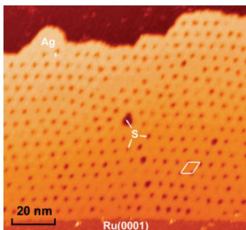
Fig. 6. S etching induced restructuring of the 1 atomic layer of Ag/Ru(0001). A new triangular symmetry of the superstructure is formed with S-filled vacancy islands 50 Å apart. [Color figure can be viewed in the online issue, which is available at [www.interscience.wiley.com](http://www.interscience.wiley.com).]
